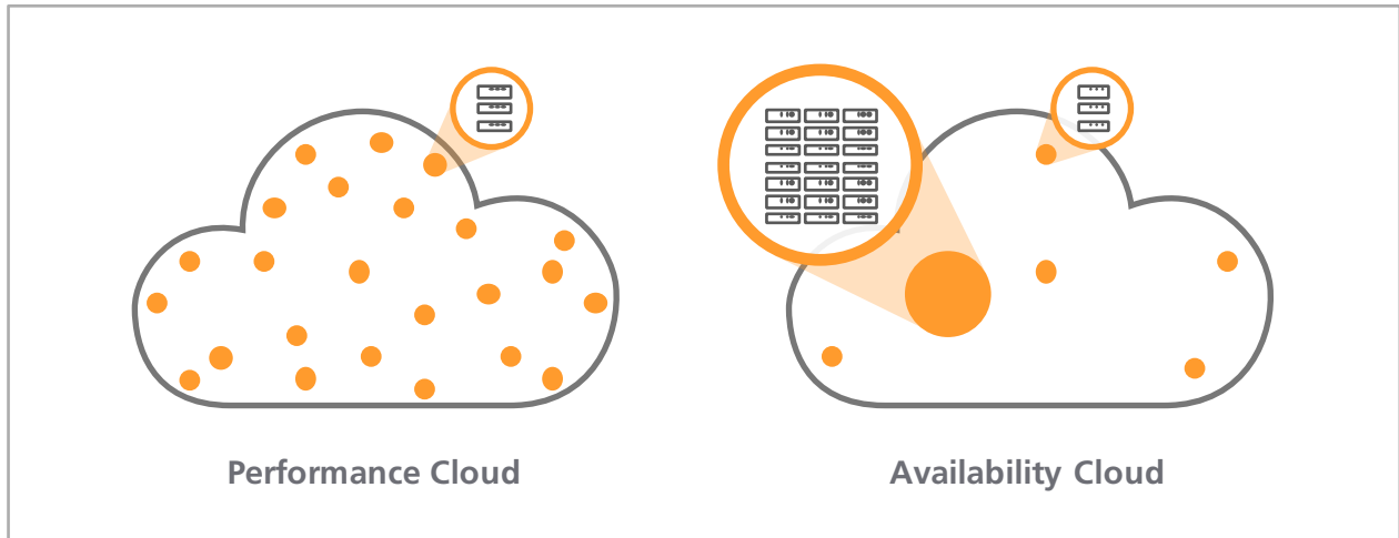
Figure 1: Fast DNS combines multiple DNS clouds with different architectures to offer an optimal combination of performance, availability and resiliency against DDoS attack.
