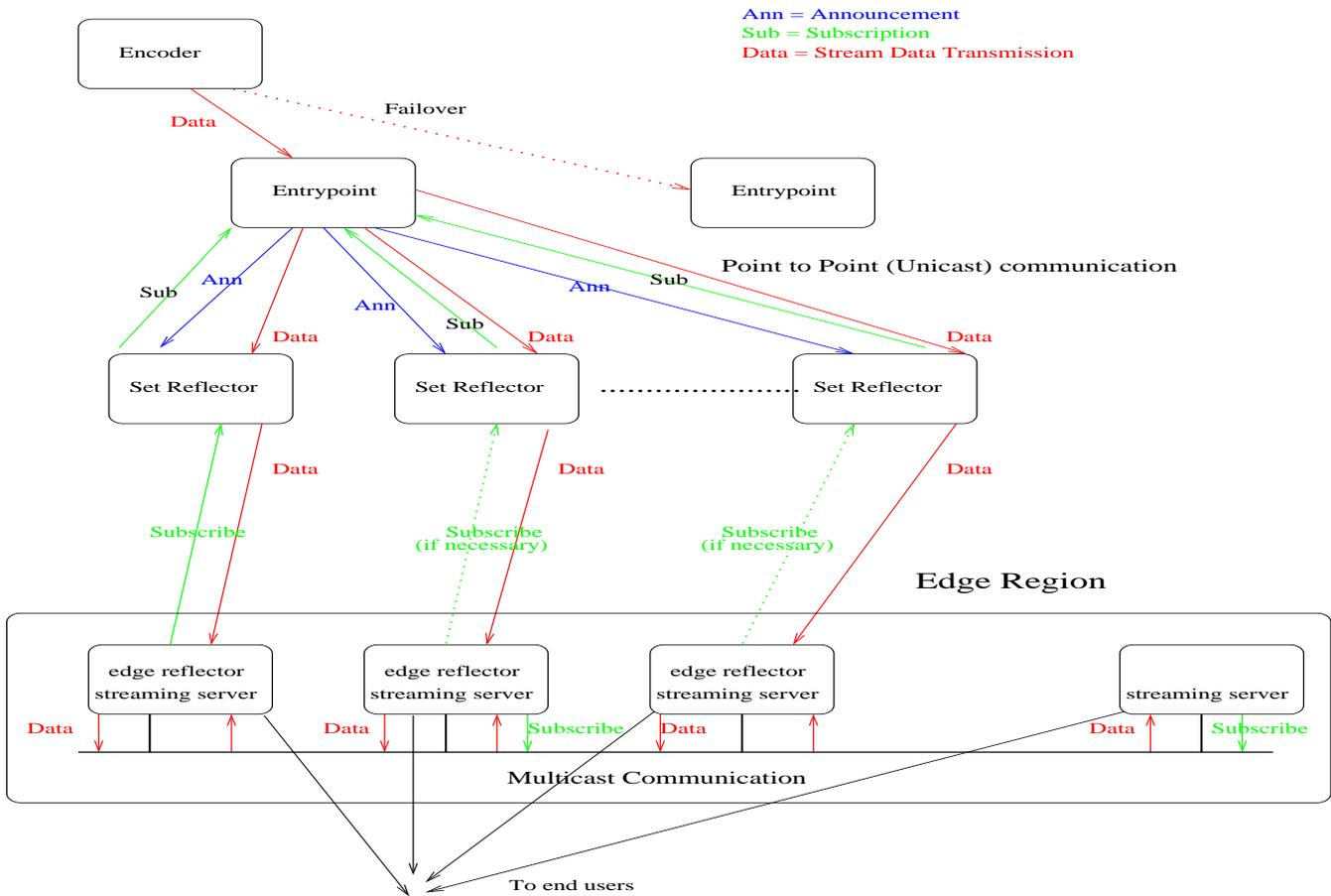
Fig. 1. High level diagram of a streaming CDN
