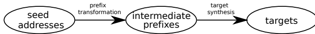
Figure 1: IPv6 topology target generation: addresses from various seeds are transformed into intermediate prefixes which are then synthesized into targets.
